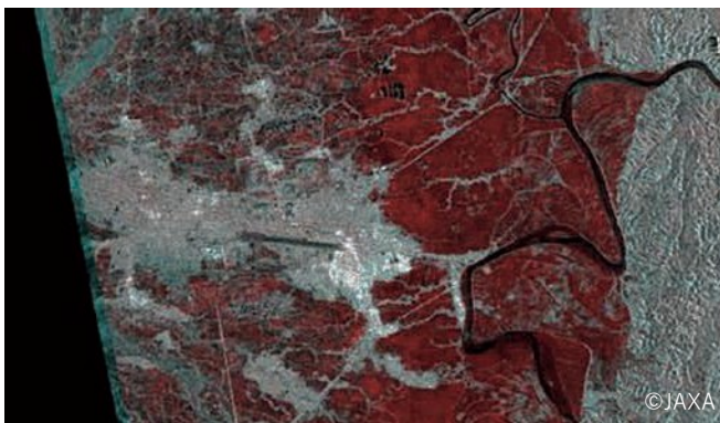
Fig. 5: Example of superimposition of images from two timings (the case of flood)
