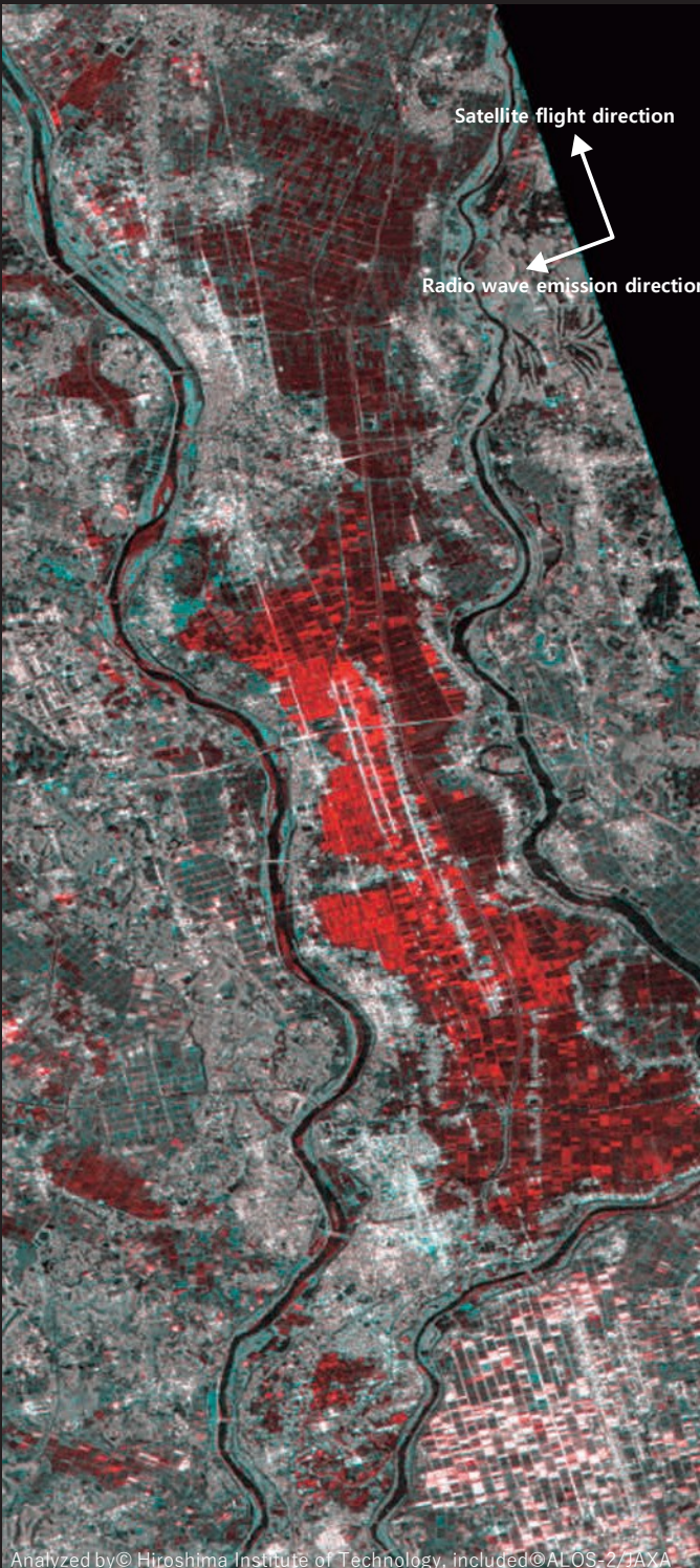
Fig. 2: Estimated flooded area extraction image by ALOS-2 (Left: enlargement of Fig. 1 Joso City, right: estimated flooded area up to 16 Sep 2015) The area of Joso City which suffered catastrophic flooding due to embankment destruction is shown enlarged in Fig. 2. It can be seen that the results are similar to the Geospatial Information Authority of Japan (GSI)'s estimated flooded area of 11 Sep 13:00 (brown). It is possible to obtain such analysis results regularly by SAR satellites such as ALOS-2 regardless of day/night or weather conditions.
